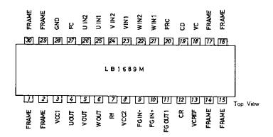
Note: All FRAME pins are connected to GND.
