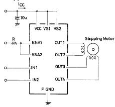
Note: Use one of the FRAME-GND pins for grounding, when the Cufoild side is soldered, heat radiation can be more improved.
