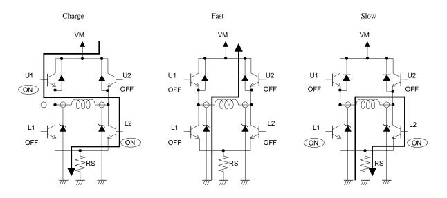
The figure above shows the current direction at PH = "H." Note that the upper diode is incorporated and the lower diode is an external Schottky diode.
