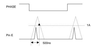
Measure the current flowing to pin E during phase switching of "H"  $\rightarrow$  "L" and "L"  $\rightarrow$  "H" after its conversion to the voltage with a detection resistor.
