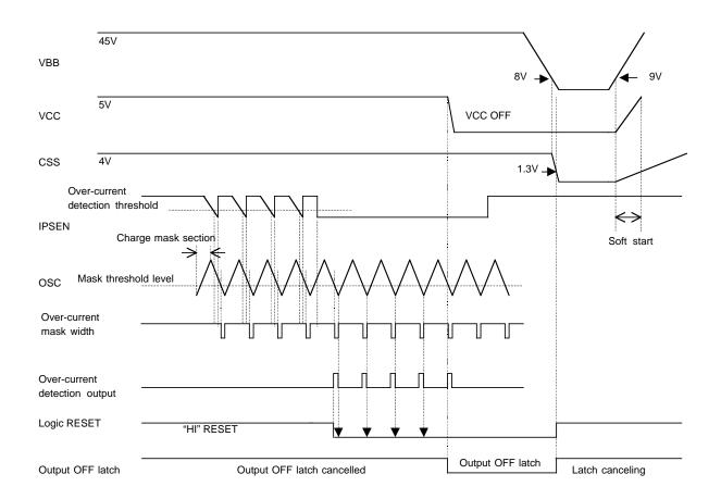
The DC/DC over-current limit value is determined from the resistor connected between VBB and current sense pin. Current limit value = 0.5(V)/RL
