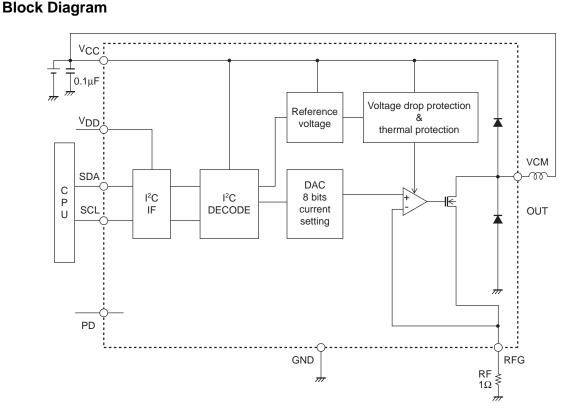
Wiring resistance (thick line) around the RF is added to the resistance of RF as an error. It must be kept as small as possible.
