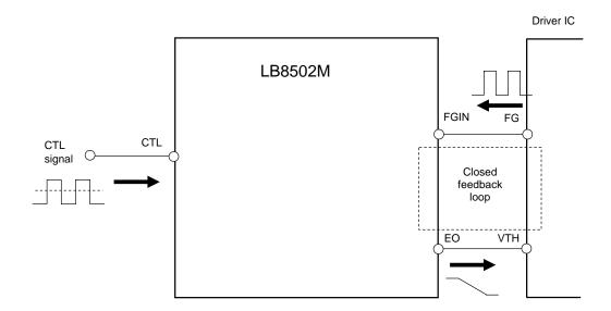
As shown in the figure below, the LB8502M generates a pulse signal from edges on the FG signal and then generates a pulse width waveform determined by the RC time constant in a one-shot multivibrator.
