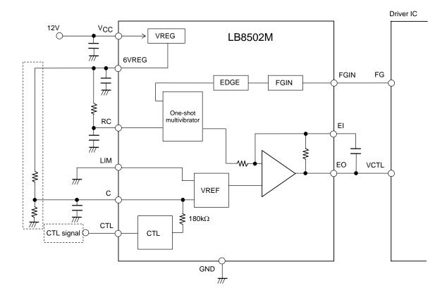
Input a fixed-duty signal to the CTL pin signal input as an input signal for which soft start is enabled at startup. Alternatively, apply a constant voltage to the C pin. (In this case, the CTL pin must be left open.)
