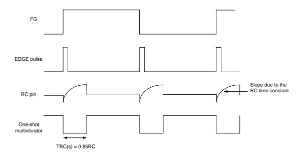
It is also possible to change the slope of the VCTL/speed relationship as shown in the speed control diagram in the previous section by changing the pulse width with the RC time constant.
