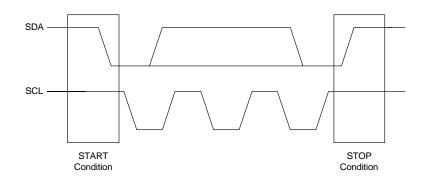
The **START condition** is recognized by the  $E^2$ PROM when a H/L edge arises on the dataline SDA during the high phase of the clock.
