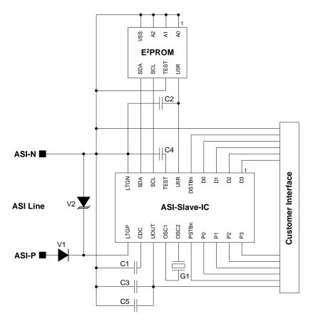
C1 = 22...470 nF / max. AS-Interface BUS DC voltage C2 = 10...220 nF / max VU5R = 5.5 V C3 = 10...470  $\mu$ F / max. (VUOUT + VUOUTp) = 29.1 V C4 = 22...100 nF / max. (VUOUT + VUOUTp + 1.4 V) = 30.5 V C5 = 10...100 nF (close to the IC) / max. (VUOUT + VUOUTp) = 29.1 V V1 = 1N4002 or equivalent V2 = TGL 41-39A or equivalent G1 = AS-Interface Crystal 5.333 MHz
