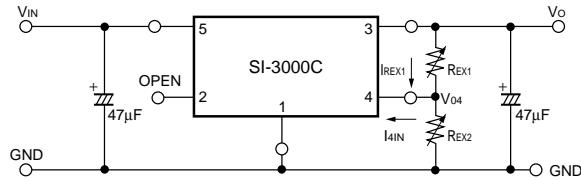
The output voltage may be increased by inserting resistors  $R_{EX1}$  between terminals No.4 (sensing terminal) and No.3 (output terminal) and  $R_{EX2}$  between terminals No.4 and No.1 (ground terminal).
