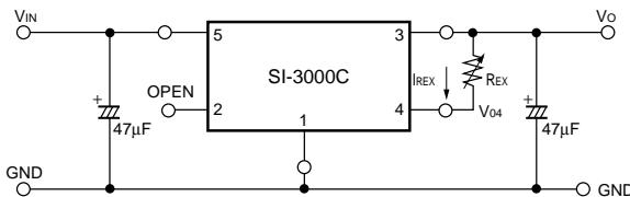
The output voltage may be increased by inserting resistor  $R_{EX}$  between terminals No.4 (sensing terminal) and No.3 (output terminal). The current  $I_{REX}$  flowing into terminal No.4 is 1mA (typ.)(SI-3033C:0.43mA (typ.)), therefore the adjusted output voltage  $V_{OUT}$  is:
