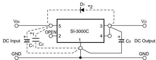
$C_0$  : Output capacitor (47 to 100 $\mu$ F)
