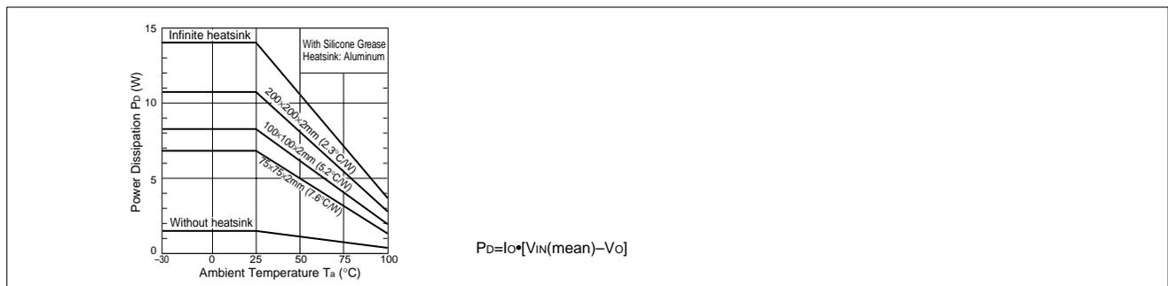
■Typical Characteristics (at  $V_o=15.7V$  for SI3025B)
