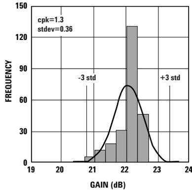
**Figure 3. Gain @ 2 GHz 3V 60 mA.**
