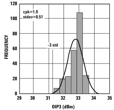
**Figure 4. OIP3 @ 2 GHz 3V 60 mA.**
