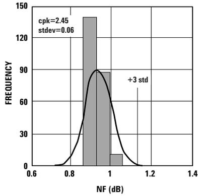
**Figure 2. NF @ 2 GHz 3V 60 mA.**
