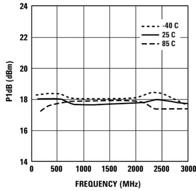
Figure 11. P1dB vs. Frequency (3V 60 mA).
