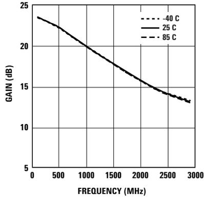
Figure 16. Gain vs. Frequency (5V 60 mA).
