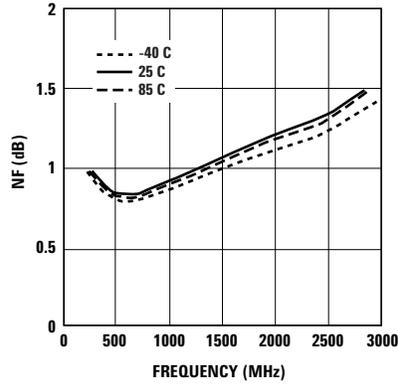
Figure 9. NF vs. Frequency (3V 60 mA).
