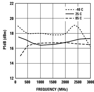
Figure 23. P1dB vs. Frequency (5V 30 mA).
