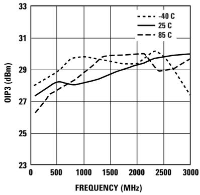
Figure 22. OIP3 vs. Frequency (5V 30 mA).
