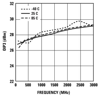
Figure 14. OIP3 vs. Frequency (3V 30 mA).
