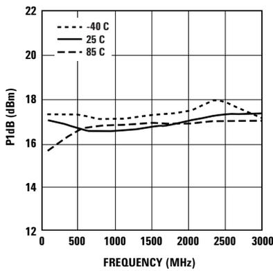
Figure 15. P1dB vs. Frequency (3V 30 mA).
