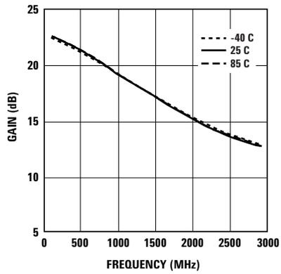
Figure 12. Gain vs. Frequency (3V 30 mA).
