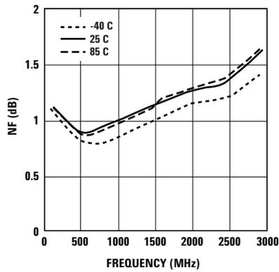
Figure 17. NF vs. Frequency (5V 60 mA).
