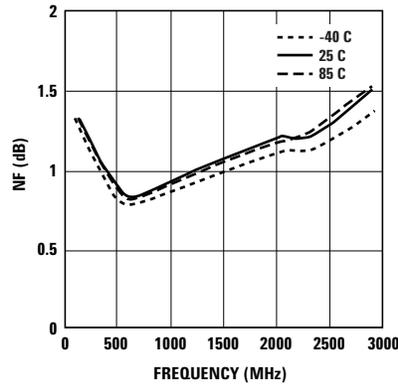
Figure 21. NF vs. Frequency (5V 30 mA).
