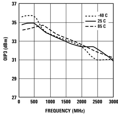
Figure 10. OIP3 vs. Frequency (3V 60 mA).
