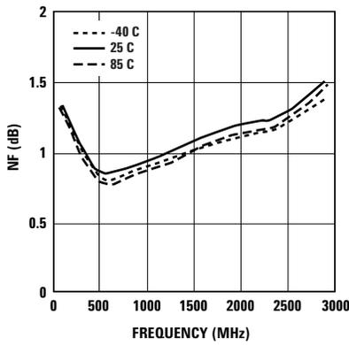
Figure 13. NF vs. Frequency (3V 30 mA).
