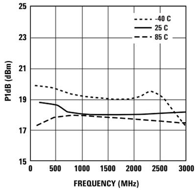
Figure 19. P1dB vs. Frequency (5V 60 mA).
