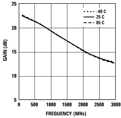
Figure 20. Gain vs. Frequency (5V 30 mA).
