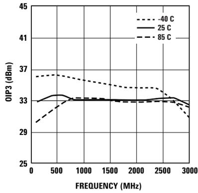
Figure 18. OIP3 vs. Frequency (5V 60 mA).
