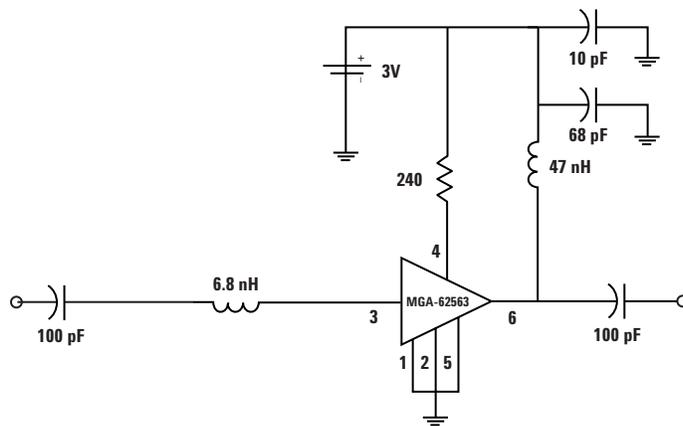
**Figure 1.** Test circuit of the 0.5 GHz production test board used for NF, Gain and OIP3 measurements. This circuit achieves a trade-off between optimal NF, Gain, OIP3 and input return loss. Circuit losses have been de-embedded from actual measurements.
