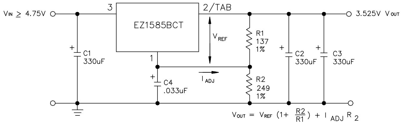
(1) C1 NEEDED IF DEVICE IS FAR FROM FILTER CAPACITORS.
