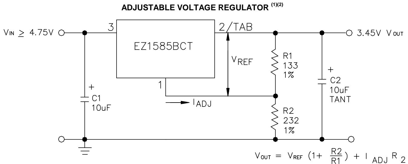
(1) C1 NEEDED IF DEVICE IS FAR FROM FILTER CAPACITORS.
