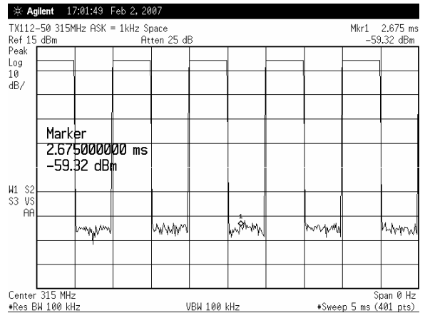
315MHz, Power Level at Space, VDD = 3.0V, ASK = 1kHz
