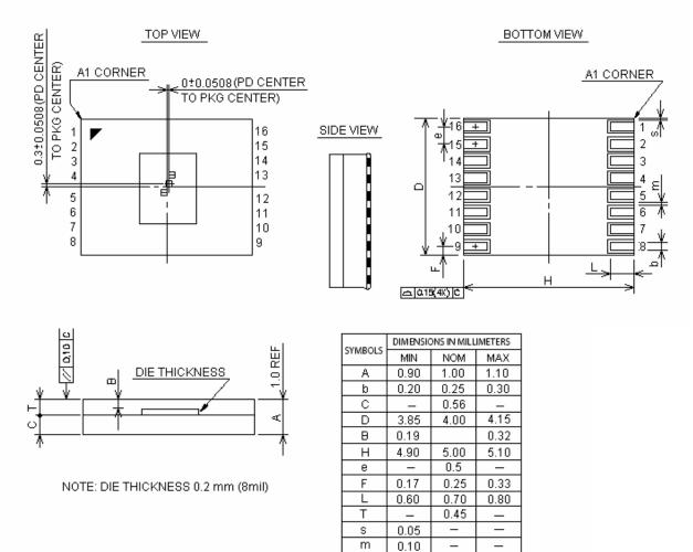
**NOTE ON DETECTOR ORIENTATION WITHIN PACKAGE:** Detector "H" is the photo detector element closest to the top of the package (closest to pins 1 and 16).
