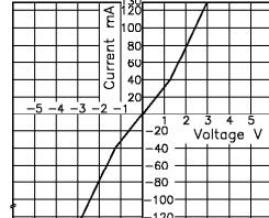
**Fig.9** Off state leakage current
