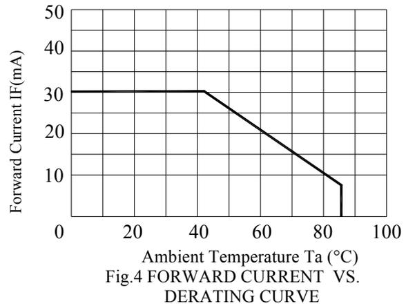
Fig.4 FORWARD CURRENT VS. DERATING CURVE
