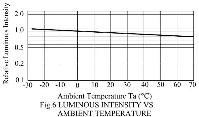
Fig.6 LUMINOUS INTENSITY VS. AMBIENT TEMPERATURE
