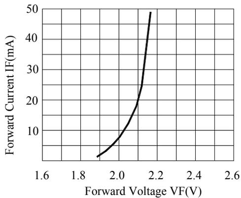
Fig.3 FORWARD CURRENT VS. FORWARD VOLTAGE PER CHIP
