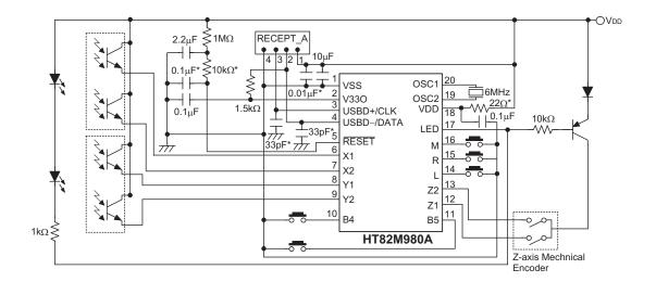
Note: Layout 0.1μF capacitor, 22Ω resistor and 0.01μF capacitor as close to VDD pin as possible.
