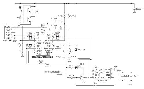
Note: \* For resistor value selection, refer to high or low input level of Z1 and Z2 in the D.C. Characteristics table. The recommended value is  $6k\Omega$ .
