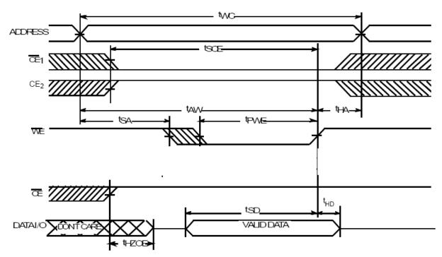
Switching Waveforms (continued) Write Cycle 2 (**CE**1 or CE2 Controlled) [9, 10, 14, 15, 16]
