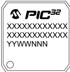
100-Lead TQFP (12x12x1 mm)
