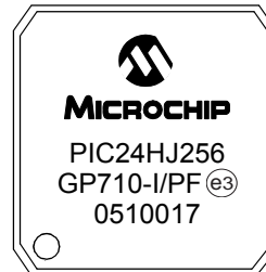
100-Lead TQFP (14x14x1mm)
