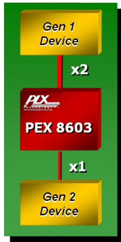
Figure 5. Gen 1 to Gen 2 Bandwidth Bridge
