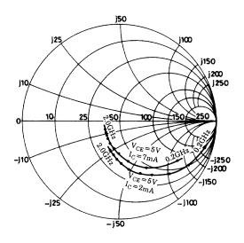
$V_{CE}\!=\!5V \\ f\!=\!200 \text{ to } 2000 \text{MHz } (200 \text{MHz Step})$
