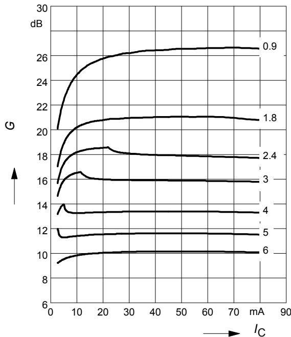
**Power gain  $G_{ma}, G_{ms} = f(V_{CE})$**
