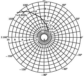
$\begin{array}{l} S_{12e} \\ V_{CE} = 8V \\ I_{C} = 5 \text{mA} \\ Ta = 25 ^{\circ}C \end{array}$
