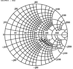
$\begin{array}{l} S_{11e} \\ V_{CE} = 8V \\ I_{C} = 20 mA \\ Ta = 25 ^{\circ}C \\ (UNIT:\Omega) \end{array}$
