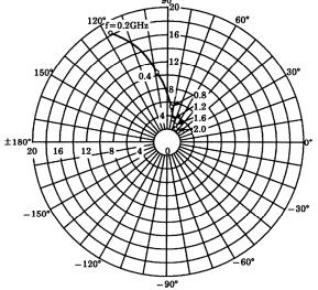
$\begin{array}{l} S_{12e} \\ V_{CE} = 8V \\ I_{C} = 20 \text{mA} \\ Ta = 25 ^{\circ}\text{C} \end{array}$
