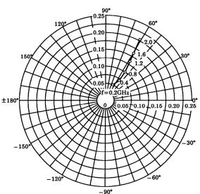
$S_{22e}$   $V_{CE}=8V$   $I_{C}=5mA$   $T_{a}=25^{\circ}C$   $(UNIT: \Omega)$
