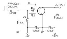
$20I_{B1} = -20I_{B2} = I_C = 300 mA$  ( ) : 2SA1319 (For PNP, the polarity is reversed.)
