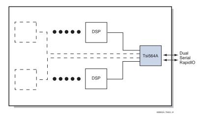
The Tsi564A provides traffic aggregation through packet prioritization when it is used with RapidIO-enabled I/O devices. When it is in a system with multiple RapidIO-enabled processors it provides high performance peer-to-peer communication through its non-blocking switch fabric.
