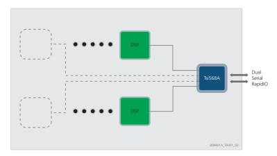
The Tsi568A provides traffic aggregation through packet prioritization when it is used with RapidIO-enabled I/O devices. When it is in a system with multiple RapidIO-enabled processors it provides high performance peer-to-peer communication through its non-blocking switch fabric.
