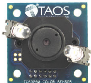
TCS3200-DB with lens, standoffs, and screws.
