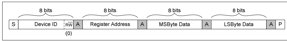
Figure 10 Single Register Write to Specified Address
