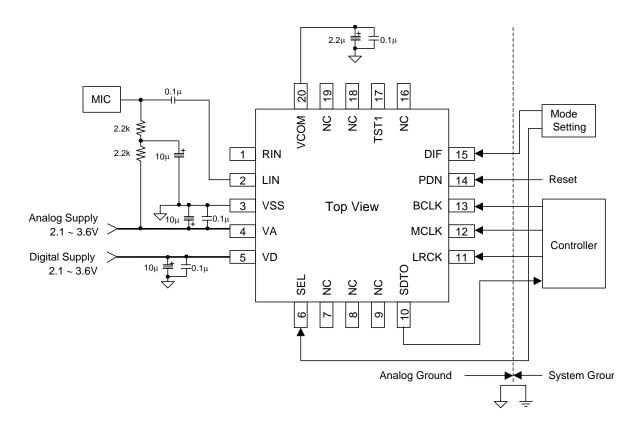
Figure 10. MIC Device Connection Example (AK5355VN)
