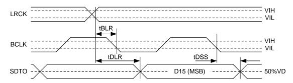
Figure 2. Audio Data Input/Output Timing (Audio I/F = No.0)
