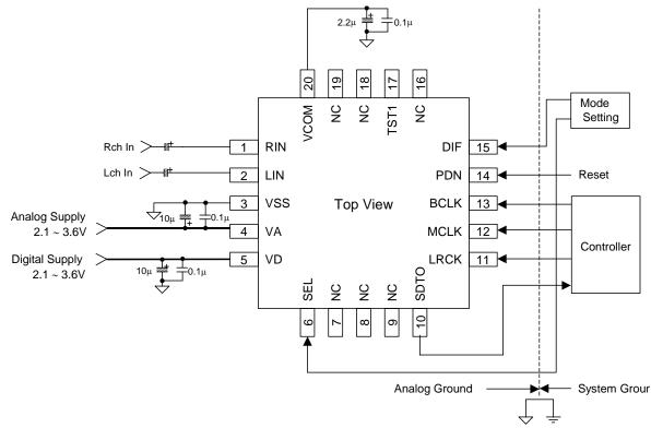
Figure 8. System Connection Diagram Example (AK5355VN)
