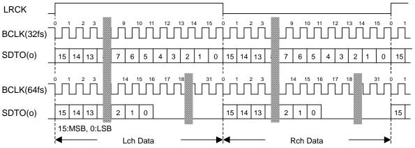
Figure 4. Audio Data Timing (No.0)
