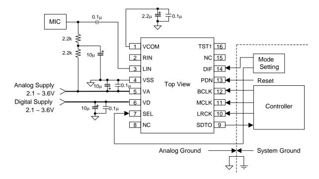
Figure 9. MIC Device Connection Example (AK5355VT)
