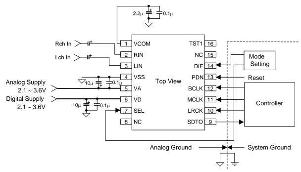
Figure 7. System Connection Diagram Example (AK5355VT)
