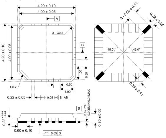
Note: The black parts of back package should be open.
