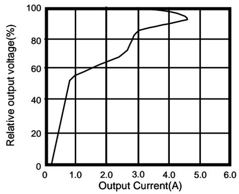
Figure 7. Overcurrent Protection Characteristics
