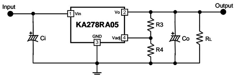
$$V_o = 1.25 \left( 1 + \frac{R_1/R_3}{R_2/R_4} \right) \quad R_1 = 1.8\text{k}\Omega, R_2 = 0.6\text{k}\Omega$$
