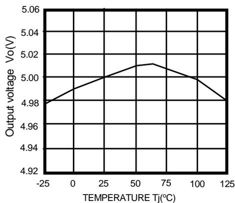
Figure 3. Output Voltage vs. Temperature( $T_j$ )
