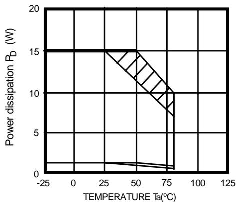
Figure 6. Power Dissipation vs. Temperature( $T_a$ )
