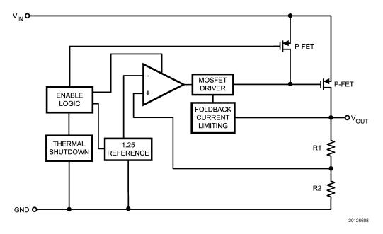
FIGURE 2. LP38690 Functional Diagram (TO-252)
