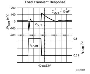
$\begin{tabular}{ll} \textbf{Typical Performance Characteristics} & \textbf{Unless otherwise specified:} & \textbf{T}_{J} = 25 ^{\circ} \textbf{C}, & \textbf{C}_{IN} = \textbf{C}_{OUT} = 10 \ \mu \textbf{F}, \\ \textbf{enable pin is tied to } & \textbf{V}_{IN} & \textbf{(LP38692 only)}, & \textbf{V}_{OUT} = 1.8 \mbox{V}, & \textbf{V}_{IN} = \mbox{V}_{OUT} + 1 \mbox{V}, & \textbf{I}_{L} = 10 \mbox{mA}. & \textbf{(Continued)} \\ \end{tabular}$
