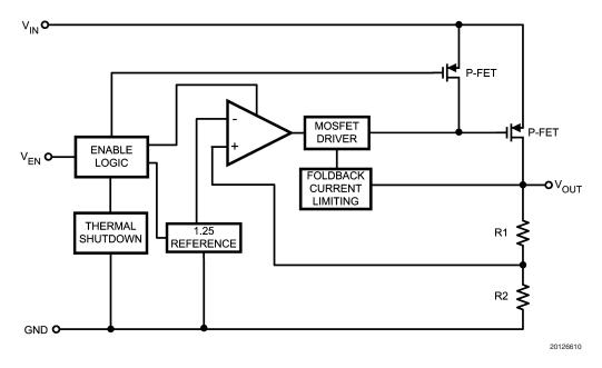
FIGURE 4. LP38692 Functional Diagram (SOT-223)
