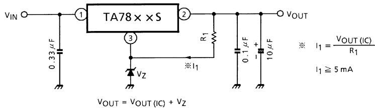
(b) Voltage boost by use of resistor
