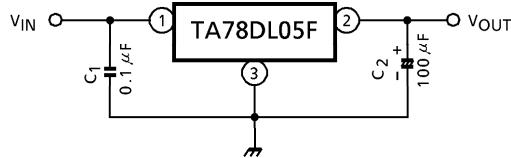
Capacitor  $C_2$  must be guaranteed to operate of the temperature range that the regulator should be operated correctly.
