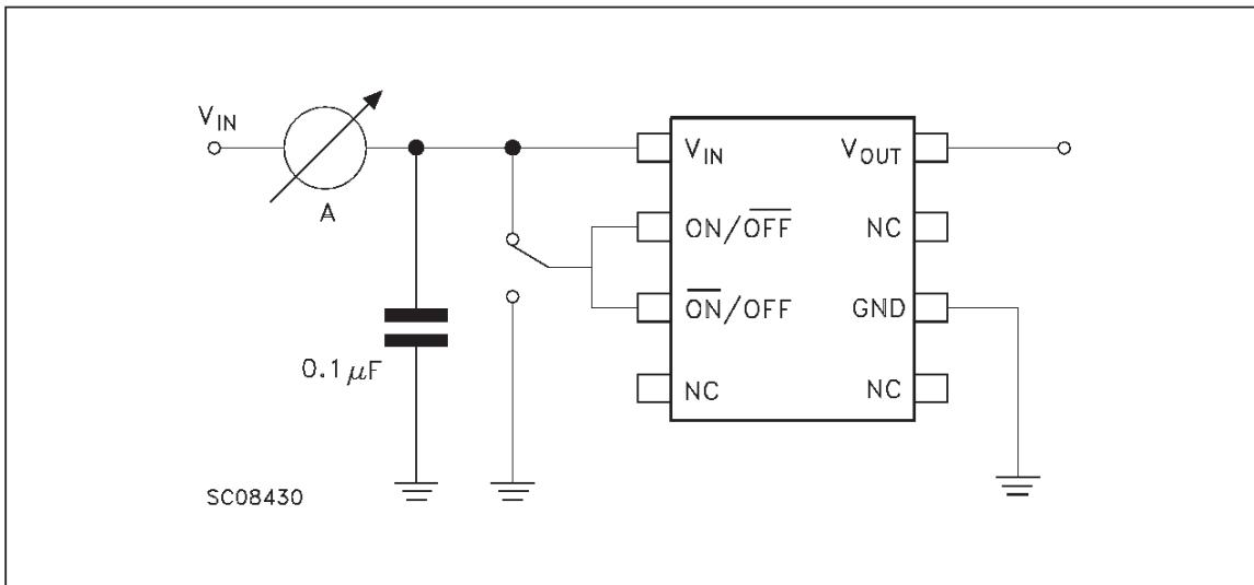
NOTE: The switch emulates the two possibilities to set the regulator in OFF mode.
