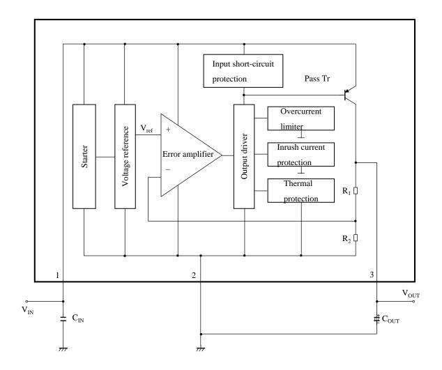
$\begin{array}{l} C_{IN} \ : \ 0.33 \ \mu F \\ C_{OUT} : \ 33 \ \mu F \end{array}$
