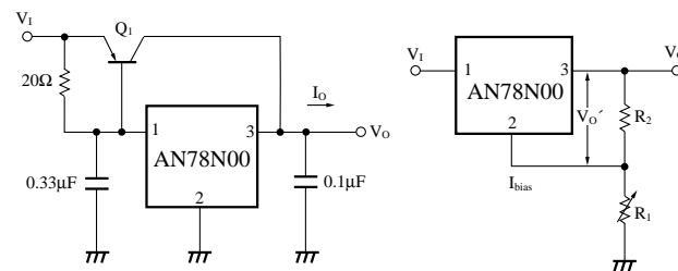
$$|V_O| = V_{O'} + \left( I_{bias} + \frac{V_{O'}}{R_2} \right) R_1$$
