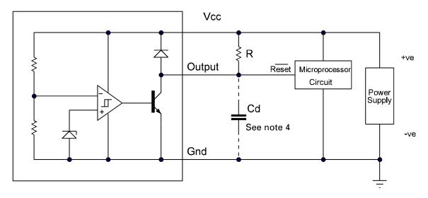
Note 4: A time delayed reset can be accomplished with the additional Cd.
