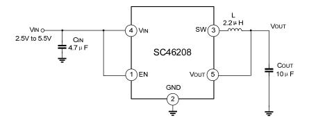
Fig.2: Output voltage fixed regulator
