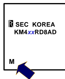
b. Top marking example of mirrored package
