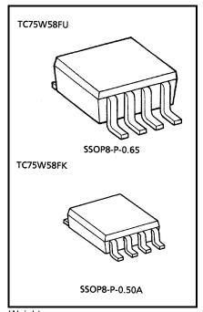
Weight SSOP8-P-0.65: 0.021g (typ.) SSOP8-P-0.50A: 0.01g (typ.)
