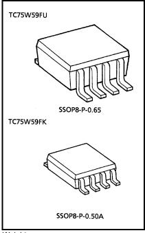
Weight SSOP8-P-0.65: 0.021g (typ.) SSOP8-P-0.50A: 0.01g (typ.)
