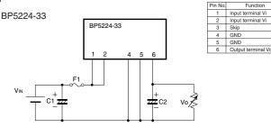
Be sure to evaluate it under the cindition that it is mounted by your product. Especially, Confirm whether output current never exceeds a maximum standard with current probe.
