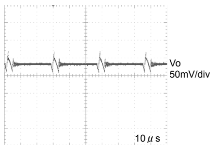
Fig.34 Output Voltage (Vo=3.3V, QLLM, Io=0A)
