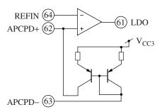
A current mirror circuit of which primary side is APCPD— is built-in. In case where output of secondary side is connected to APCPD+ and PD current for laser monitor is sunk to PD, the direction of current can be reversed by connecting the PD output to APCPD—.
