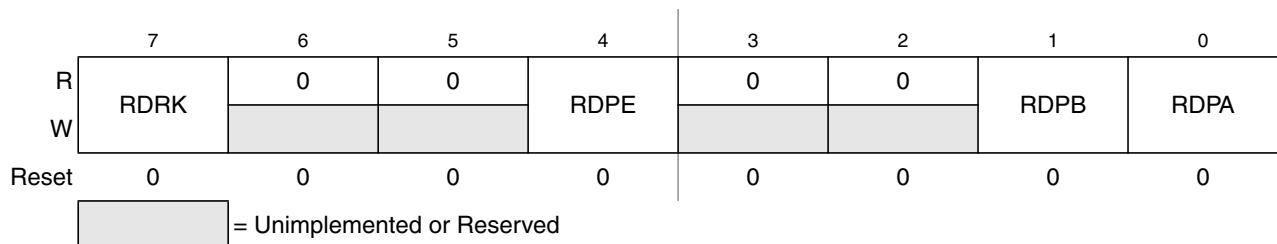
Figure 4-15. Reduced Drive Register (RDRIV)
