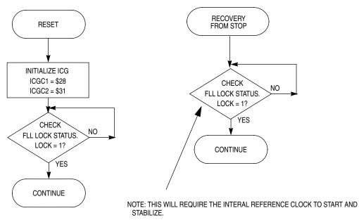
Figure 9-16. ICG Initialization and Stop Recovery for Example #3
