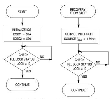
Figure 9-15. ICG Initialization and Stop Recovery for Example #2
