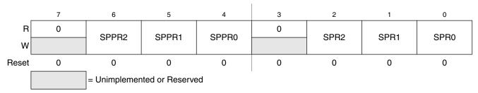
Figure 12-8. SPI Baud Rate Register (SPIBR)
