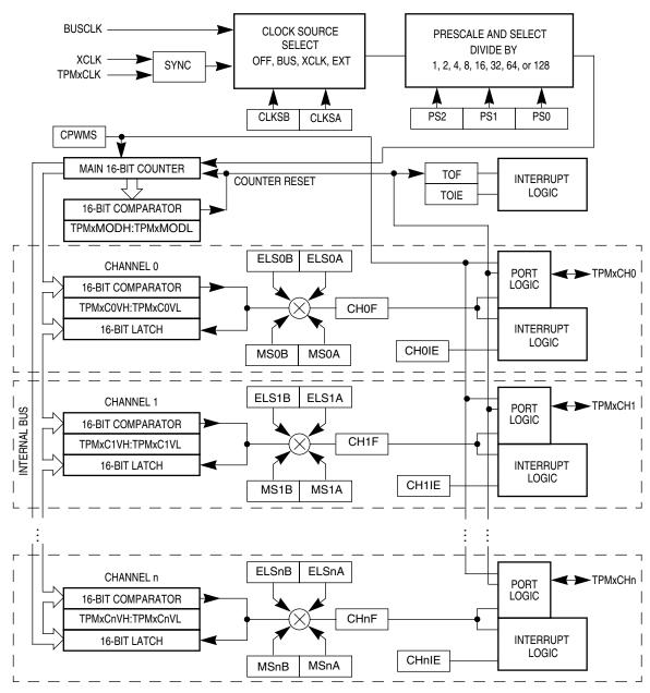
Figure 10-2. TPM Block Diagram
