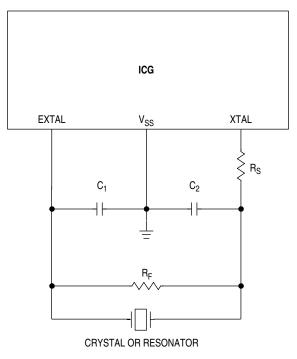
Figure 9-5. External Frequency Reference Connection
