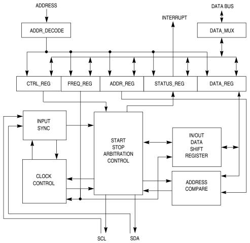
Figure 13-2. IIC Functional Block Diagram
