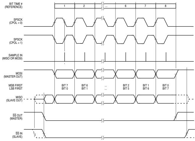
Figure 12-11. SPI Clock Formats (CPHA = 1)
