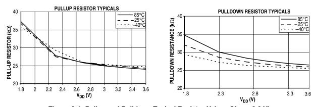
Figure A-1. Pullup and Pulldown Typical Resistor Values (V<sub>DD</sub> = 3.0 V)
