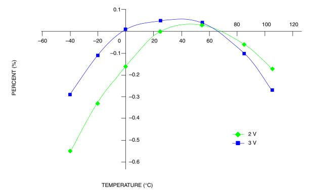
Figure A-10. Internal Oscillator Deviation from Trimmed Frequency
