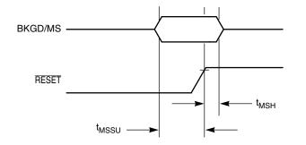
Figure A-13. Active Background Debug Mode Latch Timing
