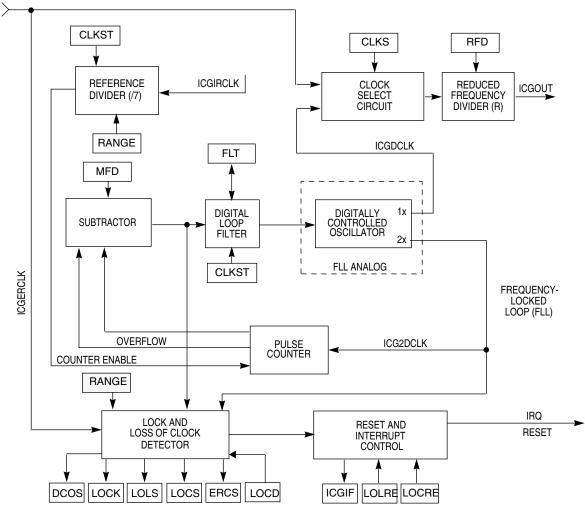
Figure 9-13. Detailed Frequency-Locked Loop Block Diagram
