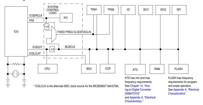
Figure 1-2. System Clock Distribution Diagram
