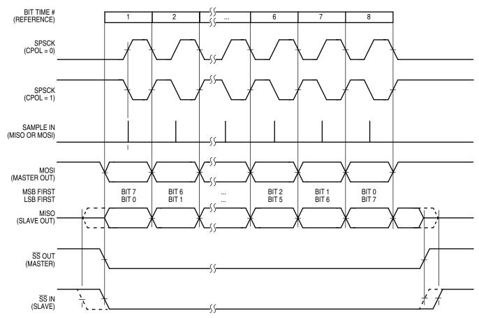
Figure 12-12. SPI Clock Formats (CPHA = 0)
