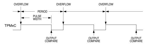
Figure 10-11. PWM Period and Pulse Width (ELSnA = 0)
