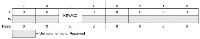
Figure 4-7. FLASH Configuration Register (FCNFG)
