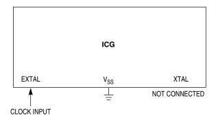
Figure 9-4. External Clock Connections
