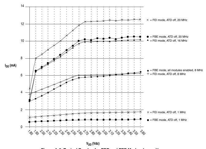
Figure A-6. Typical Run  $I_{DD}$  for FBE and FEE Modes,  $I_{DD}$  vs  $V_{DD}$
