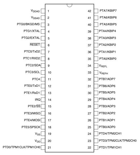
Figure 2-3. MC9S08GT16A/GT8A in 42-Pin SDIP Package
