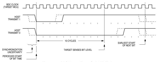
Figure 15-2. BDC Host-to-Target Serial Bit Timing
