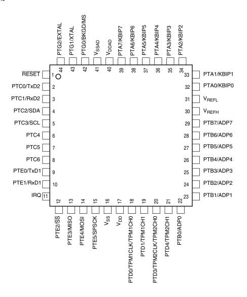
Figure 2-2. MC9S08GT16A/GT8A in 44-Pin QFP Package
