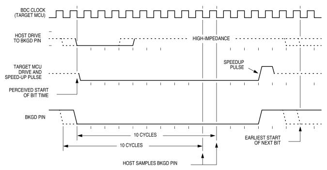
Figure 15-4. BDM Target-to-Host Serial Bit Timing (Logic 0)
