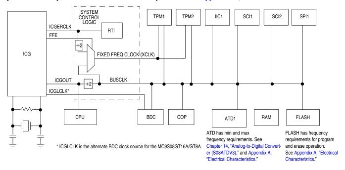
Figure 9-1. System Clock Distribution Diagram
