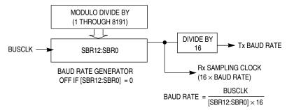
Figure 11-12. SCI Baud Rate Generation
