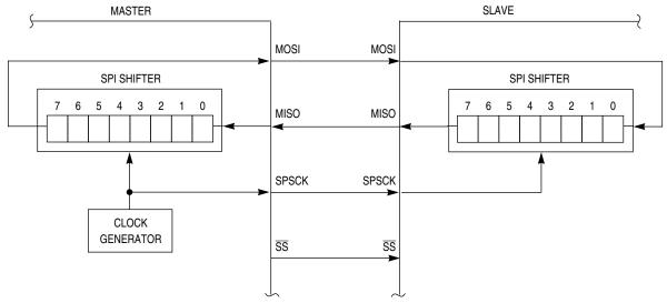
Figure 12-3. SPI System Connections
