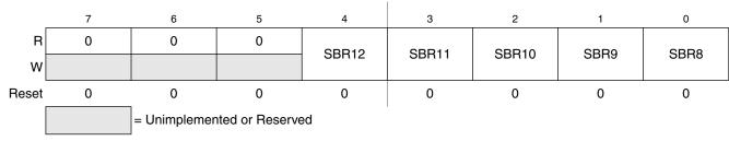
Figure 11-4. SCI Baud Rate Register (SCIxBDH)
