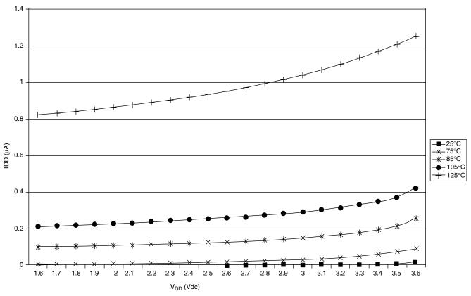
Figure A-7. Typical Stop1 I<sub>DD</sub>
