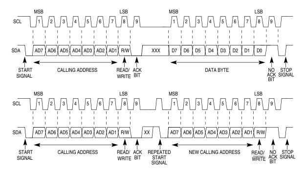
Figure 13-8. IIC Bus Transmission Signals
