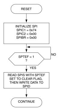
Figure 12-13. Initialization Flowchart Example for SPI Master Device
