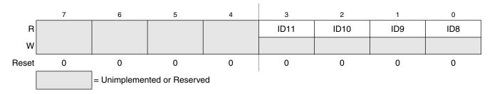
Figure 5-6. System Device Identification Register High (SDIDH)
