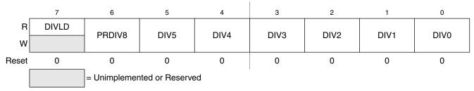
Figure 4-5. FLASH Clock Divider Register (FCDIV)
