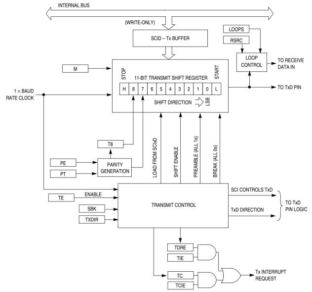
Figure 11-2. SCI Transmitter Block Diagram
