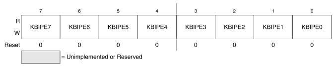
Figure 7-5. KBI Pin Enable Register (KBIPE)
