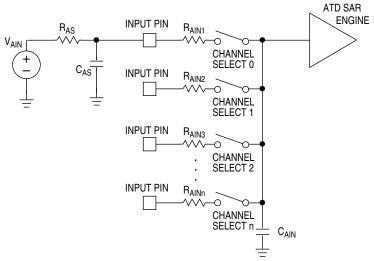
Figure 14-10. Resistor and Capacitor Placement
