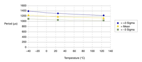
Figure A-11. Typical RTI Clock Period vs. Temperature
