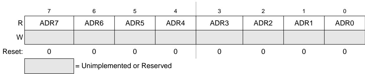
Figure 9-7. Data Result Low Register (ADCRL)
