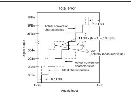
$$Total \ error \ of \ digital \ output \ "N" = \frac{V_{NT} - \{1 \ LSB \times \ (N-1) \ + 0.5 \ LSB\}}{1 \ LSB} \ \ [LSB]$$
