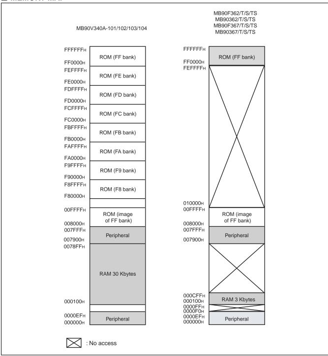
Note: The high-order portion of bank 00 gives the image of the FF bank ROM to make the small model of the C compiler effective. Since the low-order 16 bits are the same, the table in ROM can be referred without using the far specification in the pointer declaration.
