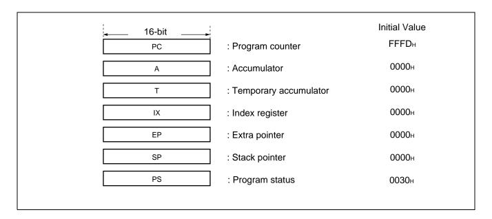
The PS can further be divided into higher 8 bits for use as a register bank pointer (RP) and a direct bank pointer (DP) and the lower 8 bits for use as a condition code register (CCR). (See the diagram below.)
