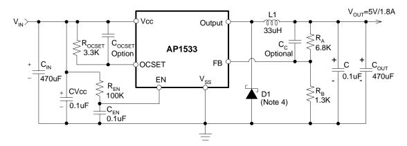
$V_{OUT} = V_{FB} x (1+R_A/R_B)$  $R_B = 0.7K\sim5K \text{ ohm}$
